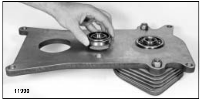
Figure 5-7. Installing Load Brake Shaft Ball Bearing in Gearcase Spider (Size 2 Hoist Shown)
