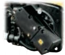
**Larger hoist drum minimizes rope wear and enhances cooling.**
