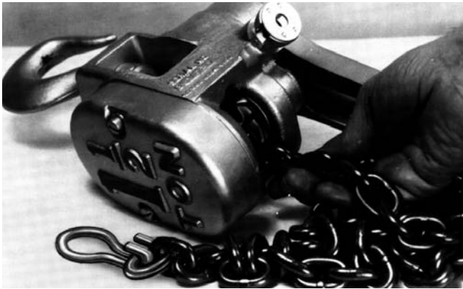
Figure 13. Chain Assembly - Hook End, 1 1/2 Ton
