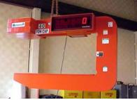
Bushman C-hooks can also be equipped with integral load weighing systems. The accuracy of the load cells is from plus or minus 0.2% to 0.5% of full load. The calibration settings are saved in memory even during loss of power. All Bushman C-hooks are designed and manufactured in accordance with ASME Spec. B30.20 and BTH-1: Design of Below-the-Hook Lifting Devices.
