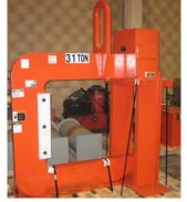
Since C-hooks are large and heavy, they can cause personal injury or property damage if they fall over. Each C-hook should be stored in an upright position on a stand specifically designed for its size, shape and weight.
