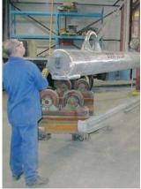
This C-hook was designed for submerging wire or rod coils in an acid pickling line. It is clad in 100% nickel to protect the steel used in the fabrication of the units.
