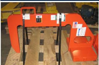
The Model 610 C-hook is similar in construction to the Model 624. The lifting bail is burned from the same piece of plate as the hook, making it an integral part of the C-hook.
