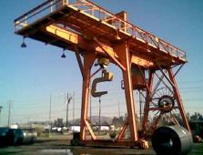
Mill duty C-hooks are built with larger sections and corner radii to keep stresses to a minimum, thereby providing maximum service life.
