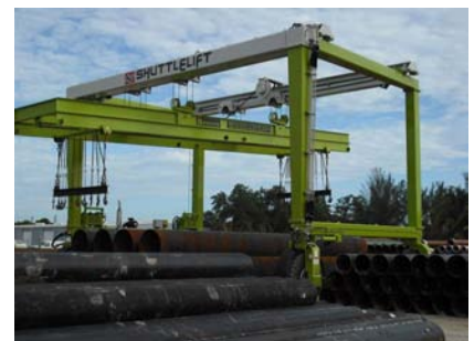
Beam with hydraulically adjustable lifting hooks
