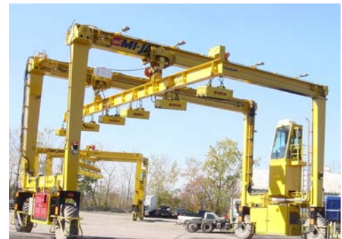
This 20-ton magnet beam attached to a mobile gantry crane has six magnets.
